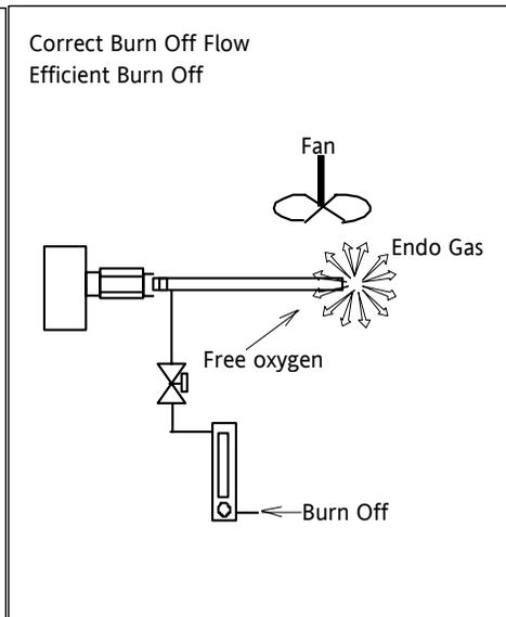
To check for the correct conditions it must be possible to convert the probe mV into percent oxygen, the table below is a guide at 927°C:
